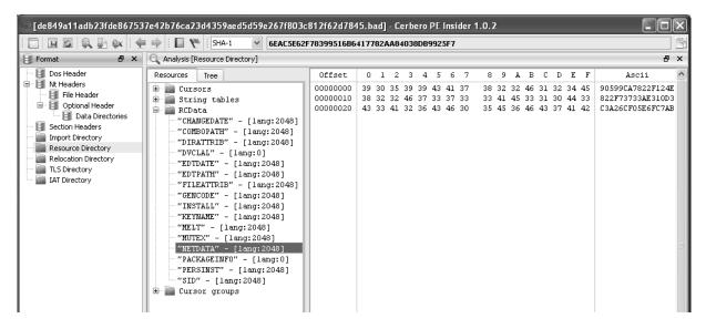
Figure 3.5: DarkComet version 4 binary showing configuration information.
