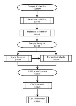
Figure 4.10: Message queue process flow.
