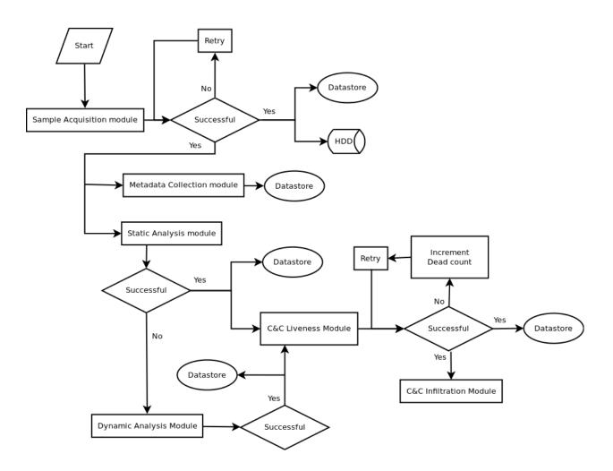
Figure 4.1: Framework process flow.
